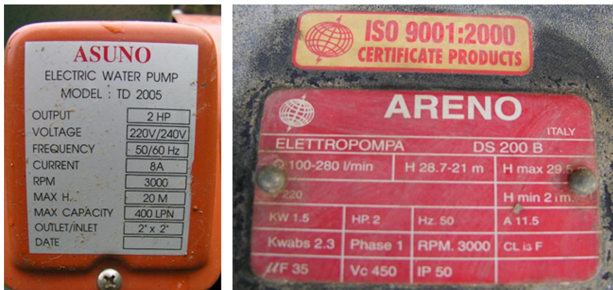
Figure 9: Example for the signboard with technical data of a motor-pump-combination
