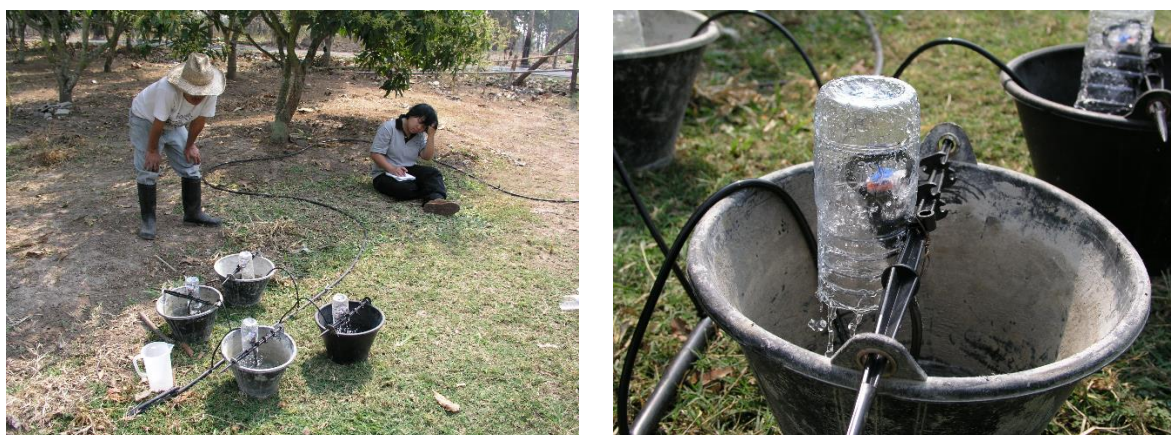
Figure 14: Field testing of micro-sprinklers (left); a cut-open water bottle enables to capture all the water from a micro-sprinkler into a bucket (right)
